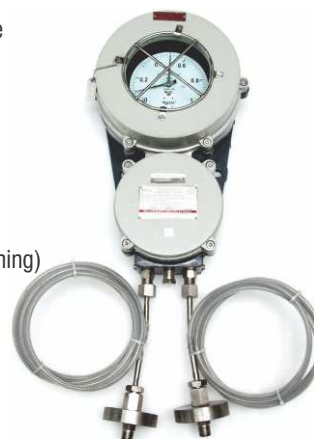
Bellow type, with Micro switch, Flame proof Case & Diaphragm Seal
