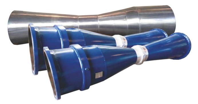
**General** Venturi Tubes serve users with accurate measurement of non-viscous fluids in clean & dirty streams. Venturi Tubes are virtually maintenance-free and corrosion-resistant. Venturi tubes are manufactured in strict accordance with ASME MFC-3M, BS-1042 and ISO-5167 standards. These measurement standards provide users with +/-1.0% uncertainty of discharge coefficient. For critical measurement applications, wet calibration at reputed flow laboratories can be offered.
